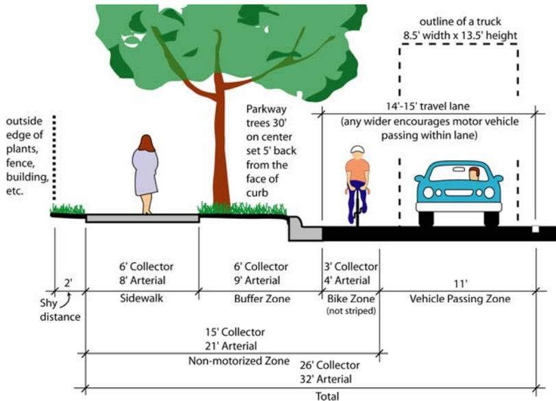
In this scenario, there are no specifically designated bicycle facilities within the roadway. Bicycles are accommodated through increased right-hand lane width (14' to 15') and reduced traffic speeds. Education and enforcement programs along with signage and potential pavement markings, such as the Shared-use Arrow, are utilized to alert motorists to the bicyclist's presence in the roadway.
