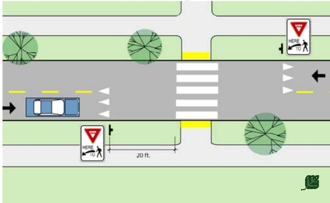
“Yield Here to Pedestrians” signs and yield line pavement markings should be placed a minimum of 20 ft. in advance of a crosswalk to encourage drivers to stop a greater distance from the crosswalk.
