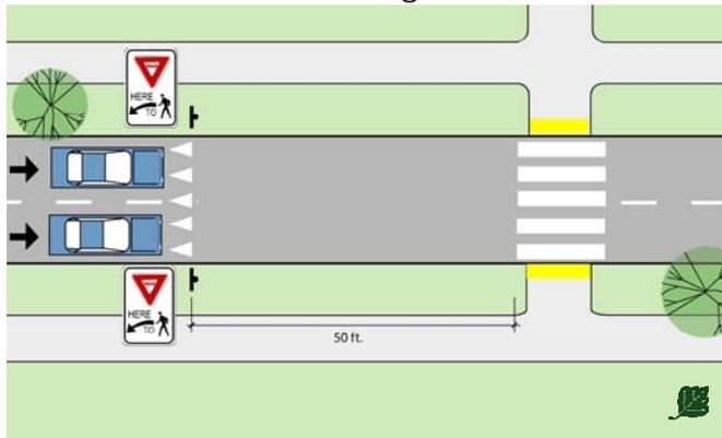
“Yield Here to Pedestrians” signs and yield line pavement markings should be placed further in advance of a crosswalk on multi-lane roads to minimize the risk of a multiple-threat crash (see illustration in this section) and provide improved visibility for motorists in adjacent lanes.
