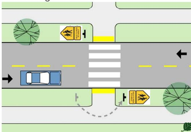
“Yield Here to Pedestrians” signs should be placed on either side of the road to ensure visibility for motorists in both lanes.
