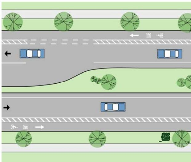
This striped buffer is replaced with a dashed line where bicycle-merging movements are expected.
