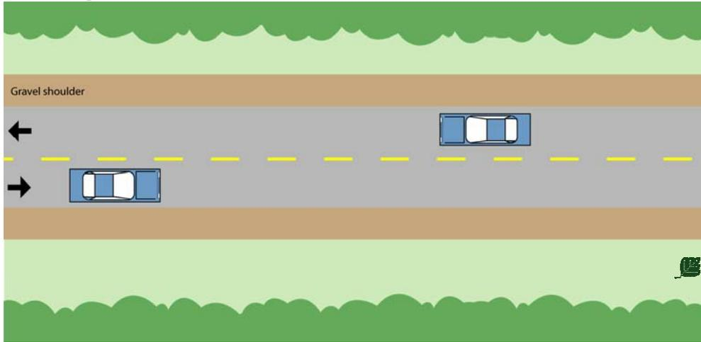
A rural cross-section (no curbs) with gravel or grass shoulder. The existing roadway travel lanes are not of a sufficient width to accommodate bicycle lanes by lane narrowing.
