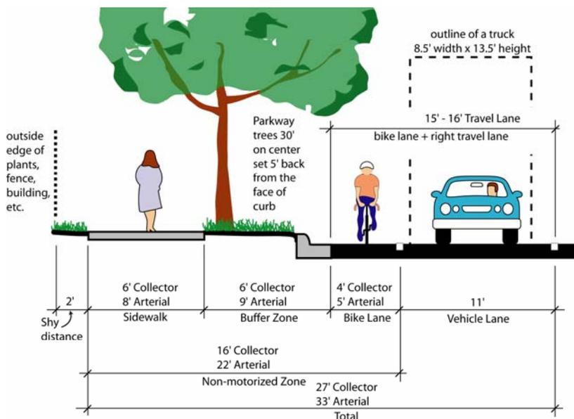
In this scenario, striped bicycle lanes or designated paved shoulders are provided on all collectors and minor arterials. Principal Arterials may have bike lanes or widened curb lanes, as determined most prudent for specific situations. The width of the bicycle lanes or shoulders should increase in areas with poor sight lines and/or higher vehicular speeds and volumes.
